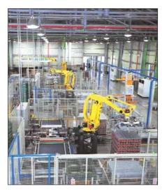
For aerosol top and bottom domes, Clevertech installed three wrapping machines connected to two joined snake palletisers. The equipment details were developed jointly with the technical team at Sun Group, and the system operates at up to 500 ends a minute, per infeed.
